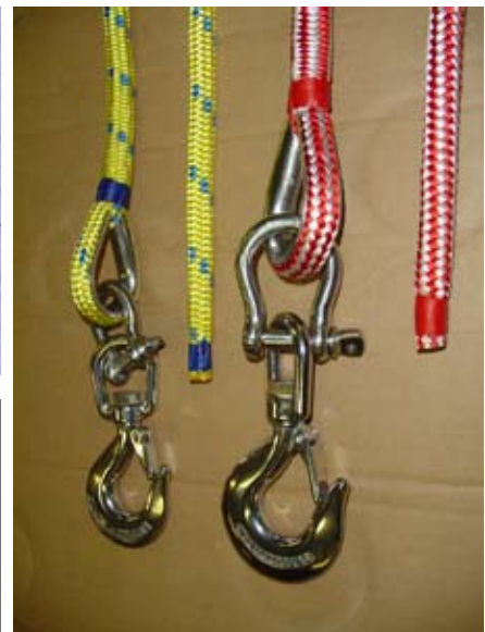
Above - Stainless steel thimble splice with a premium quality quick release snap shackle. Pull on the clasp to open the torsion bail. If your line is subject to twisting, then we recommend the use of a hook that is on a bearing. Make connections to your boat's bow eye using such a hook. Right - 1/2" & 5/8" lines with appropriately sized swivel eye hooks and anchor shackles.
