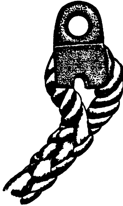
Figure 582-10-3 Thimble and Link.
